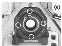
② Put the "Lock Ring Tool for X-2 Finder Unit" on the retaining ring so that 「pins」 of the Lock Ring Tool seat in the slots [(b ①)] and slowly turn it counterclockwise to remove the retaining ring [(b ②)][(c)]. Then pull the pre-installed 45°Viewfinder out carefully not to damage "O-ring contact surface" of the X-2 rear body[(d)].
