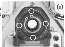
② Put the "Lock Ring Tool for X-2 Finder Unit" on the retaining ring so that 『pins』 of the Lock Ring Tool seat in the slots [(b ①)] and slowly turn it counterclockwise to remove the retaining ring [(b ②)][(c)]. Then pull the pre-installed Straight Viewfinder out carefully not to damage "O-ring contact surface" of the X-2 rear body[(d)].
