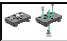
To attach optional accessories to the "Quick Shoe Plate UWTP-QB1", remove the M2 Cap Bolts and/or Tripod Screw (1/4-20 UNC) as required. Use the included 3/16" and 1.5 mm Allen wrenches.
