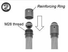
Screw *Reinforcing Ring* on the M28 thread part.
