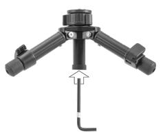
Insert the provided 3/16" Allen wrench into the elevator tube.
