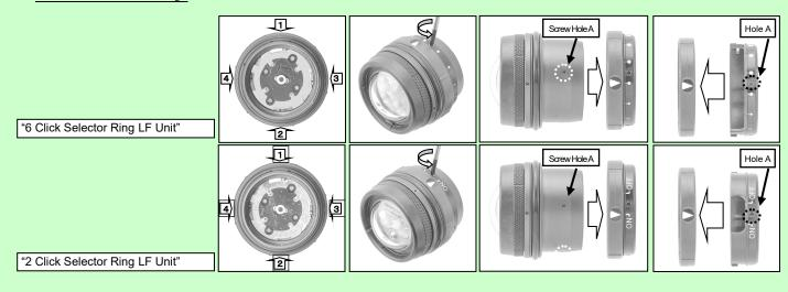
Step ② Clean to remove old grease, sands/iron sands from the "Selector Ring LF" and "Fixing Ring LF". Then check the protruded part on the "Fixing Ring LF" if it gets worn.
