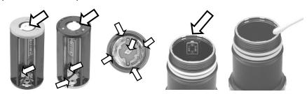
If above step fails to recover expected performance, conduct following maintenance on terminals (4 points) of the "LF1100h-EWf Light Head".
