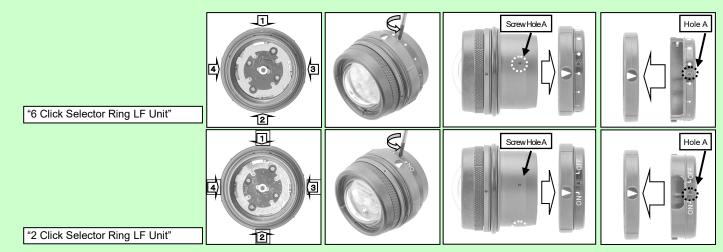
Step ② Clean to remove old grease, sands/iron sands from the "Selector Ring LF" and "Fixing Ring LF". Then check the protruded part on the "Fixing Ring LF" if it gets worn.
