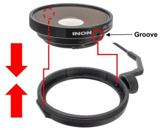
③ Secure the Focus Stick and the lens with the Focus Stick retainer. Screw the Focus Stick retainer onto the Focus Stick threads with holding the Focus Stick and lens not to slip out of the groove of the lens barrel. Be careful not to overtighten the Focus Stick retainer.
