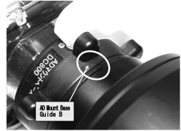
It is necessary to fill the space between UFL-165AD and housing port with water, so attach UFL-165AD underwater or partially unscrew the lens allowing inside air to escape then retighten.
