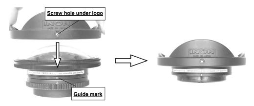
Place the lens on a flat desk and lightly and evenly tighten hollow screws diagonally by supplied Allen Wrench. <u>Too much or uneven</u> <u>tightening will damage the lens hood.</u>
