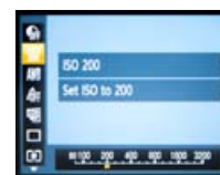
Press [FUNC./SET Button] to select ISO menu and choose desired ISO speed by [◀▶ Button].
